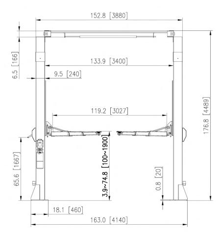
Please note, this blueprint shows the height extension kit on the LTPO15 lift. Overall height without the height extension kit is 157". This lift must be sold WITH the height kit.
