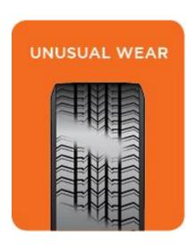
**Mechanical parts** problems can cause cupping, spotting, feathering or scalloped wear because the tire isn't tracking straight.
