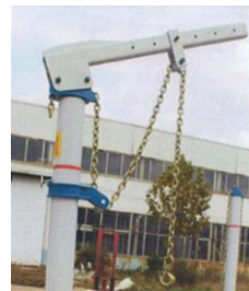
OH boom pull tower extension
